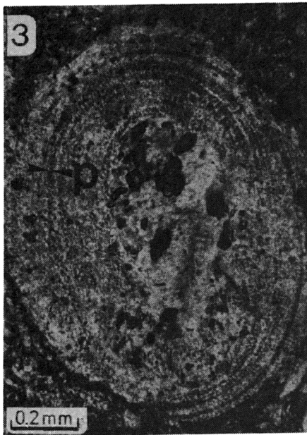
1-4 — Gypsum ooids showing concentric bands formed by: i) concentric Becke lines between zones of low refractive indices ( p in Figs 1—2), ii) dense radial Becke lines ( p in Figs 3—4); bands laterally disappear, coalesce (Figs 2—4) and cut each other (Fig. 1; arrowed ), in the latter case indicating regeneration of ooid ( n marks its nucleus); calcite crystals ( dark ) are placed within nuclei (numerously in Fig. 4), form envelopes (Fig. 4, top ) and are scattered ( c in Figs 2, 4) between bands formed by Becke lines; ooid in Fig. 3 is abraded or dissolved; in Figs 2, 4 — eccentric; polarized light; parallel (Figs 2—4) and partly crossed nicols (Fig. 1); oblique illumination (Fig. 2)
