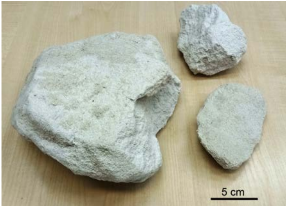
Text-fig. 7. Samples of cemented fluvial sand collected for laboratory tests (air-dry condition).
