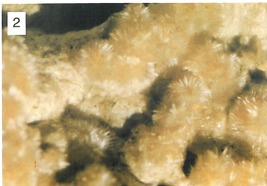
1 — Fibrous, asbestos-like crystals of fibroferrite with grains of copiapite ( arrowed ), \times 30 2 — Encrustation of fibroferrite covered by rosettes of acicular pickeringite, \times 15
