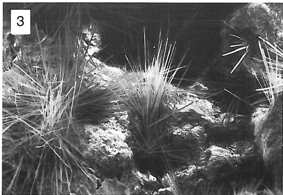
1-2 — Acicular pickeringite on copiapite; SEM, \times 200 3 — Bunches of pickeringite needles on the schist surface; SEM, \times 150
