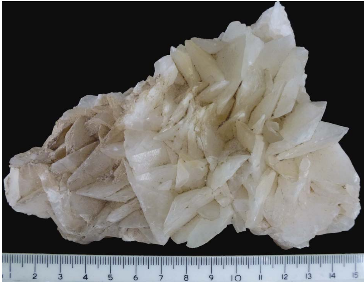
Text-fig. 23. Encrustation of large calcite crystals from an open joint in the Chalk of Selwick Bay, Yorkshire. Scale in cm
