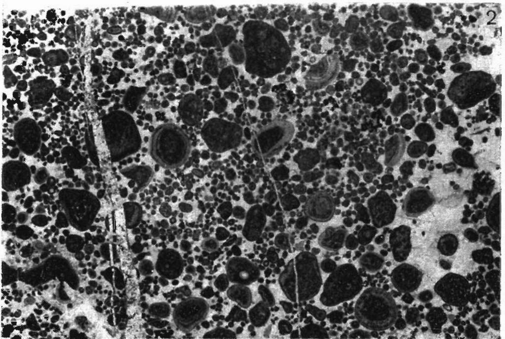
1 — Well sorted oointrasparite, in places with broken or regenerated ooids and lumps; Dalnia, Famennian;  $\times 7$ .
