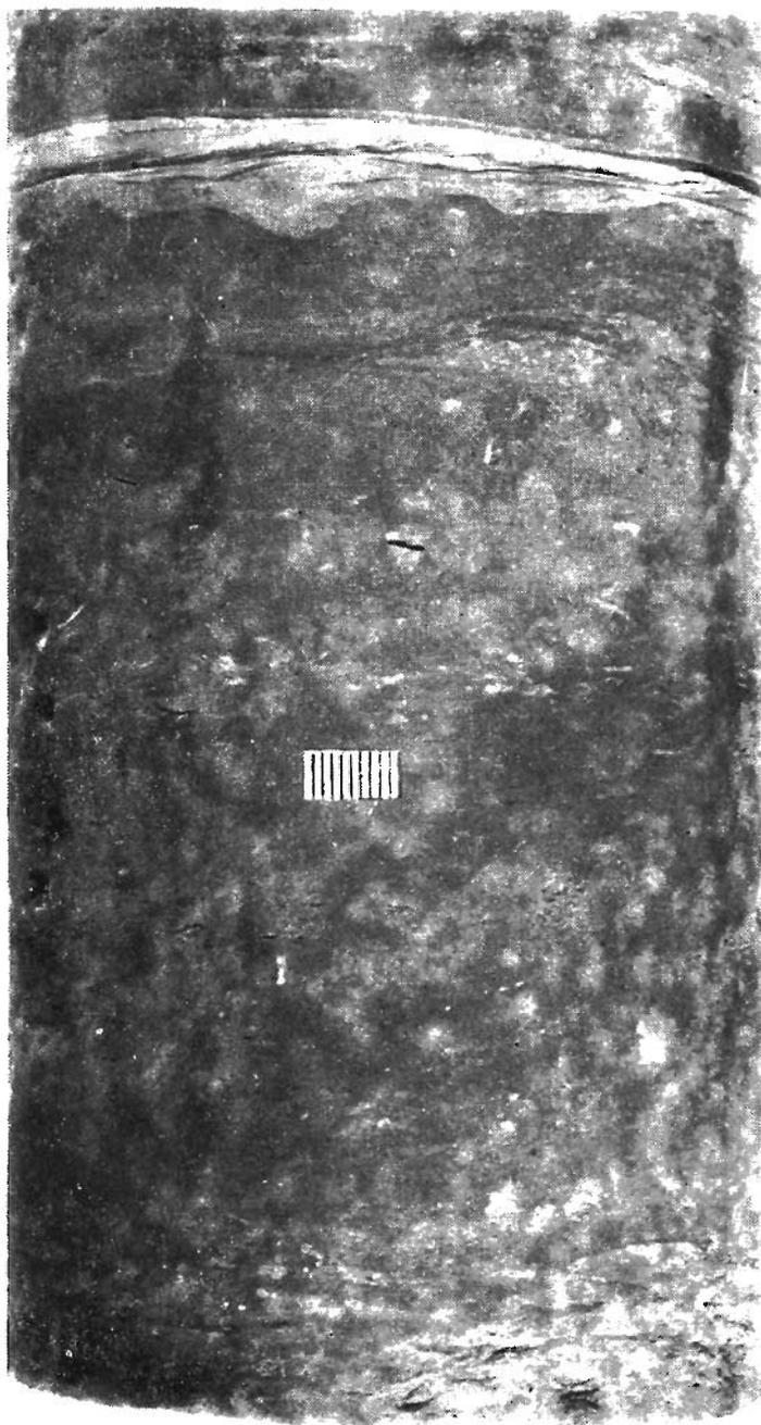
Bed of clayey siltstone here and there showing traces of cloudy structure and small shale fragments. At top a thin siltstone bed with clay intrusions at bottom Lębork (2257.0 m)
