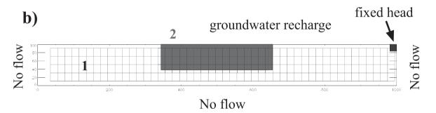
Fig. 5. b - Model scenario used for the simulations with the initial conduit network and the two regions marked as 1 and 2
