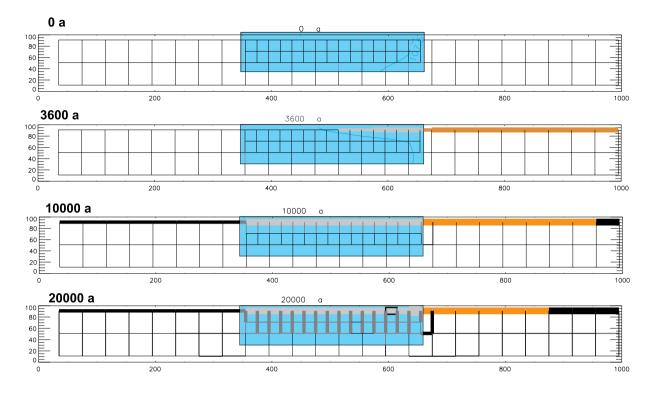
Fig. 9. Model results for Scenario 4. Now region 2 has the higher hydraulic conductivity than region 1; deep karstification is initiated in the region of higher fracture density (region 2); for legend see Fig. 6
