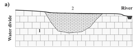
Fig. 5. a – Vertical cross section through a small catchment area; the river is to the right, a water divide to the left and in the middle a region of different hydraulic conductivity, marked as region 2, is embedded in the limestone (region 1); flow direction is from left to right; b – Model scenario used for the simulations with the initial conduit network and the two regions marked as 1 and 2
