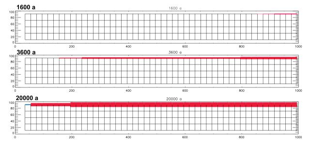
Fig. 6. Model results for Scenario 1, depicting the conduit network after 1600 a, 3600 a and 20000 a, respectively. Line thicknesses represent conduit diameters of >0.0005 m, >0.005 m, >0.01 m, >0.1 m, >0.2 m and >0.3 m, respectively. A shallow watertable cave develops
