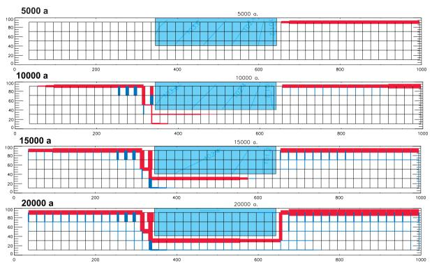
Fig. 7. Model results for Scenario 2. Around the zone of reduced hydraulic conductivity a deep phreatic cave evolves; for legend see Fig. 6
