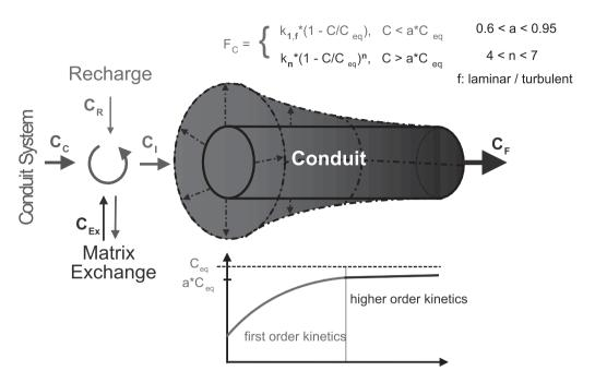
Fig. 4. Chemistry of CAVE demonstrated at one node and tube. Water coming from recharge, the upstream conduit system and the fissured system with the corresponding concentrations  $C_R$ ,  $C_C$  and  $C_{Ex}$  is mixed instantaneously and given to a conduit tube with initial concentration  $C_I$ . A possible concentration profile along the tube is depicted as well, with a\* $C_{en}$  the switching concentration from first to higher order kinetics
