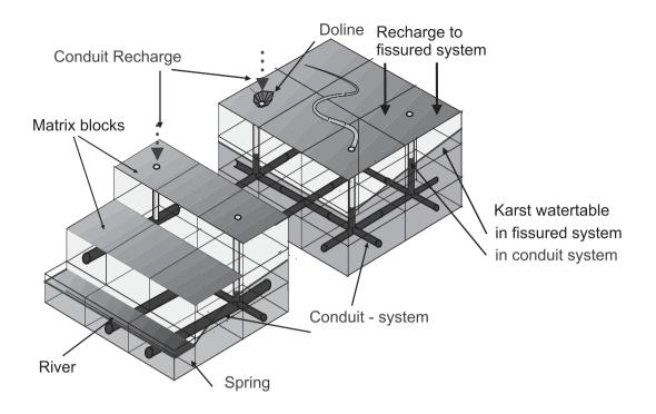
Fig. 2. Schematic representation of the hydraulic aspects of the dualistic model concept of a karst aquifer; a typical spring catchment and its representation in the numerical model CAVE is depicted
