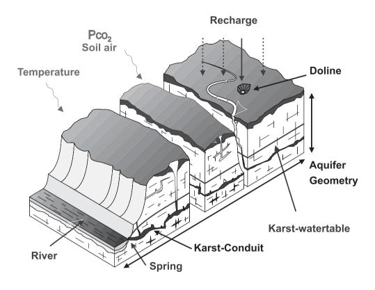
Fig. 1. Major factors influencing the genesis of a karst aquifer (schematically): geological conditions and climatic parameters
