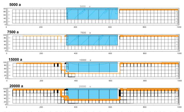
Fig. 8. Model results for Scenario 3. Deep karstification is initiated around the region of lower fracture density and thus hydraulic conductivity; for legend see Fig. 6
