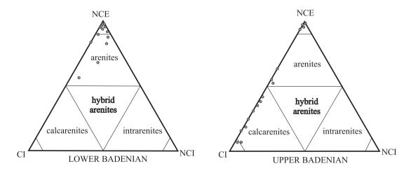
Fig. 6. NCE/NCI/CI diagram for arenites: NCE – non-carbonate extrabasinal grains; NCI – non-carbonate intrabasinal grains; CI – carbonate intrabasinal grains
