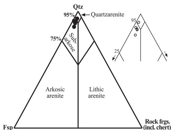
Text-fig. 4. Framework grain composition of the Jerzmanice sandstones from the North Sudectic Basin. Classification diagram after Pettijohn *et al.* 1987. Fsp – feldspars; Qtz – quartz; Rock frgs. – rock fragments
