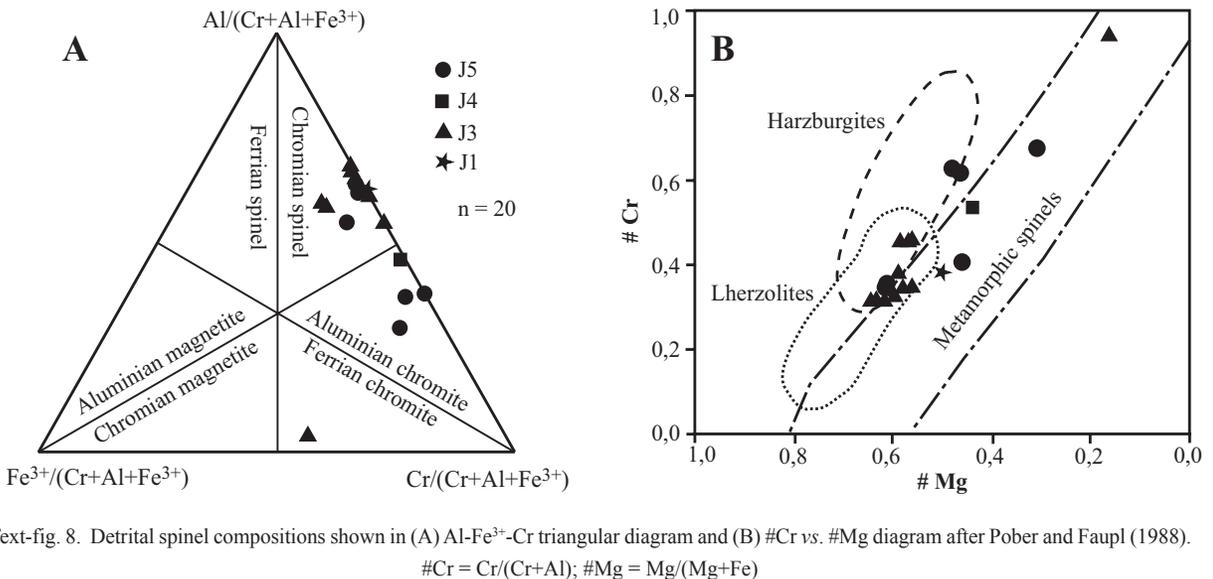
Text-fig. 8. Detrital spinel compositions shown in (A) Al-Fe<sup>3+</sup>-Cr triangular diagram and (B) #Cr vs. #Mg diagram after Pober and Faupl (1988). #Cr = Cr/(Cr+Al); #Mg = Mg/(Mg+Fe)
