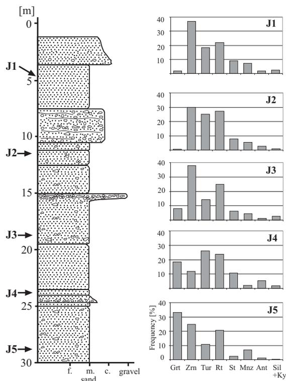
Text-fig. 3. Measured section at Jerzmanice with sample locations. Frequency diagrams show the quantitative diversity of translucent heavy minerals. Grt – garnet; Zrn – zircon; Tur – tourmaline; Rt – rutile; St – staurolite; Mnz – monazite; Ant – anatase; Sil+Ky – sillimanite and kyanite
