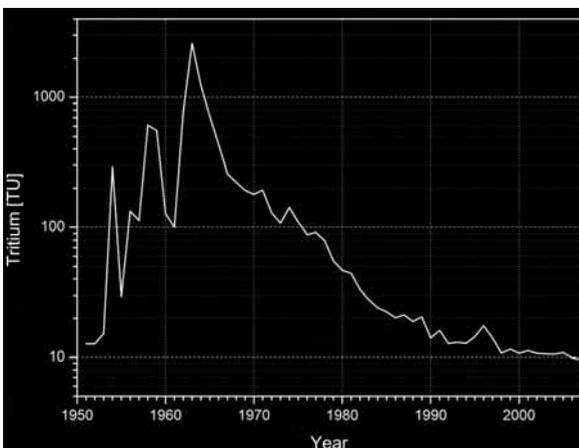
Text-fig. 14. Tritium input function used in modelling by FLOWPC code
