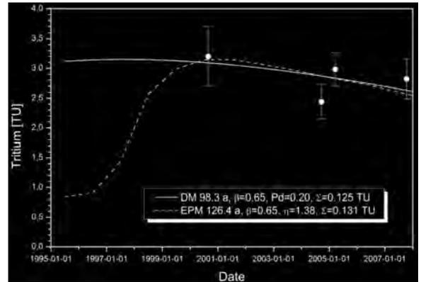
Text-fig. 23. Tritium data and fitted models, sulphate mineral water horizon in well 5p, Sokołowsko, the Sudetes Mts., Poland
