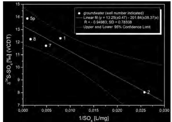
Text-fig. 8. The  $\delta^{34}\text{S-SO}_4$  as a function of reciprocal of the sulphate concentration in groundwater
