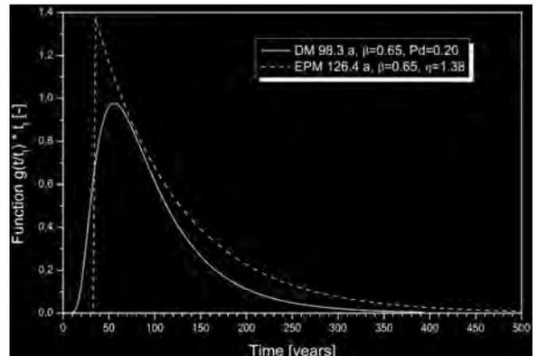
Text-fig. 24. Residence time distribution function for sulphate mineral water horizon in well 5p, Sokołowsko, the Sudetes Mts., Poland (obtained from the FLOWPC code)
