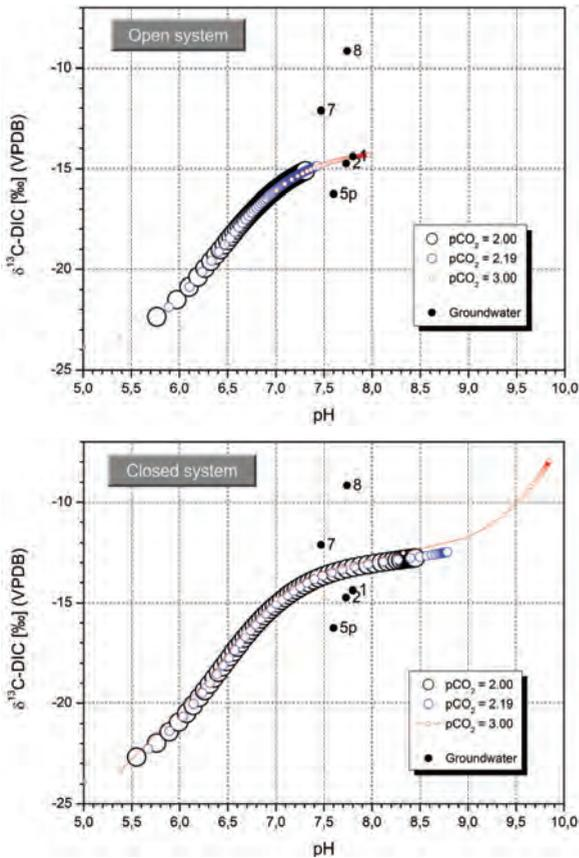
Text-fig. 9. Evolution of  $\delta^{13}\text{C-DIC}$  in groundwater during equilibration with calcite, under conditions of open (Text-fig. 9A) and closed (Text-fig. 9B) systems, at different  $\text{CO}_2$  contents. Well number indicated
