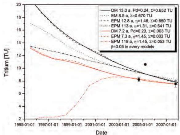
Text-fig. 17. Tritium data and fitted models, well 1, Unisław Śląski, the Sudetes Mts., Poland. Models fitted to all measurements in groundwater are marked in black, whereas models for two, lower values noted during the summer half-years marked in red
