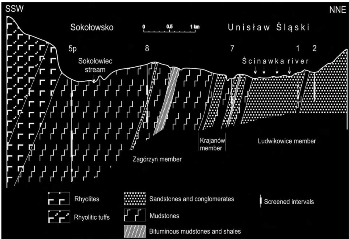
Text-fig. 2. Schematic geological cross-section (after Dobrzyński 2007a). Data on water tables, confined and piezometric surfaces met during drilling are given in Table 1
