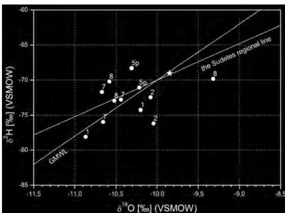
Text-fig. 4. Stable hydrogen versus oxygen isotopic composition in groundwater. The Sudetes regional line ( $\delta^2\text{H} = 5.2176 \delta^{18}\text{O} - 17.82$ ) after Ciężkowski and Kryza (1997). GMWL – global meteoritic water line,  $\delta^2\text{H} = 8 \delta^{18}\text{O} + 10$  (after Craig 1961). Star indicates average composition of Holocene infiltration waters in foreland of the studied part of the Sudetes after d'Obyrn *et al.* (1997)
