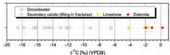
Text-fig. 11. Stable carbon isotopic composition of DIC in groundwater and carbonate mineral phases. Isotopic composition of the carbonates is given in Table 7
