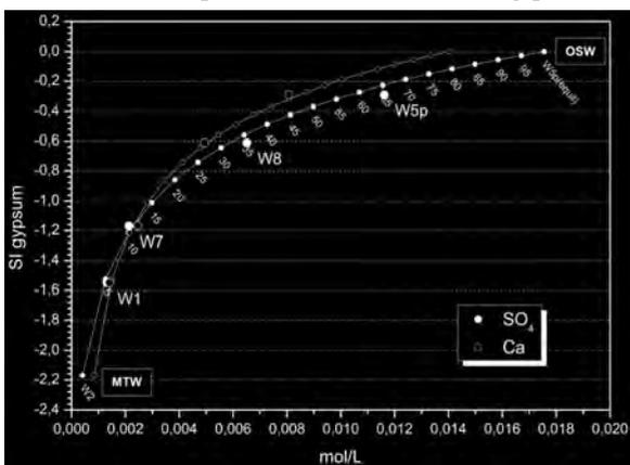
Text-fig. 13. Saturation index (SI) for gypsum vs. Ca and  $\text{SO}_4$  concentration compared with the results of water mixing modelling (after Dobrzyński 2007b). Explanations: MTW – modern tritium-bearing water, OSW – old sulphate water; W1, W2, W7, W8, W5p – sampled wells; W5p(equil) – sulphate mineral water from well 5p equilibrated with gypsum (the OSW component); 5 ÷ 95 – percentage of the OSW component
