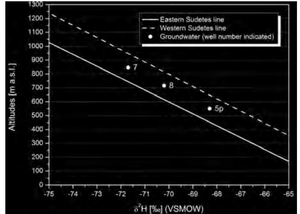
Text-fig. 5. Stable hydrogen composition of groundwater in summer compared with the Sudetic isotopic altitude curves after Ciężkowski and Kryza (1989)
