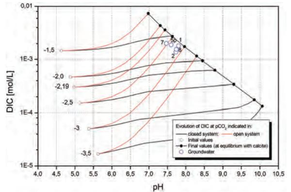
Text-fig. 10. Evolution of DIC concentration in groundwater during equilibration with calcite, under conditions of open and closed systems, and different  $\text{CO}_2$  concentrations. Well number indicated
