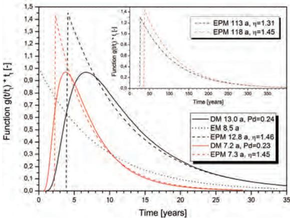
Text-fig. 18. Residence time distribution function for well 1, Unisław Śląski, the Sudetes Mts., Poland (obtained from the FLOWPC code). Models fitted to all measurements in groundwater are marked in black, whereas models for two, lower values noted during the summer half-years marked in red
